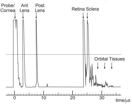
Use the information in the diagram to calculate the lens thickness. The spike labelled 'Ant Lens' corresponds to the front of the lens and the spike labelled 'Post Lens' corresponds to the back of the lens. The velocity of ultrasound in the lens is 1640 m s<sup>-1</sup>. [3]
