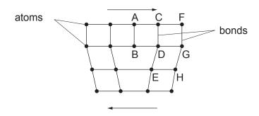
(i) Using the letters in the diagram, explain how plastic deformation takes place in ductile metals when forces are applied as shown by the arrows. Space is provided so that you can illustrate your answer if you wish to do so (or you may add to the existing diagram).
