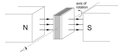
The second diagram is a 2D representation of the coil looking along the axis of rotation.
