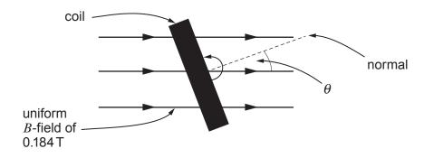
(a) (i) Calculate the flux **linkage** of the coil for the angles  $\theta = -10^{\circ}$  and  $\theta = +10^{\circ}$ . [2]
